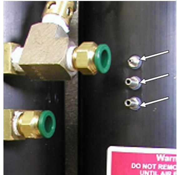
Fig. 8 Remove barbs on air tank
