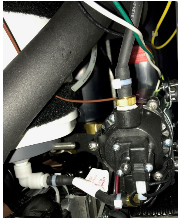
Fig. 9 Connecting black purge hose to suction canister
