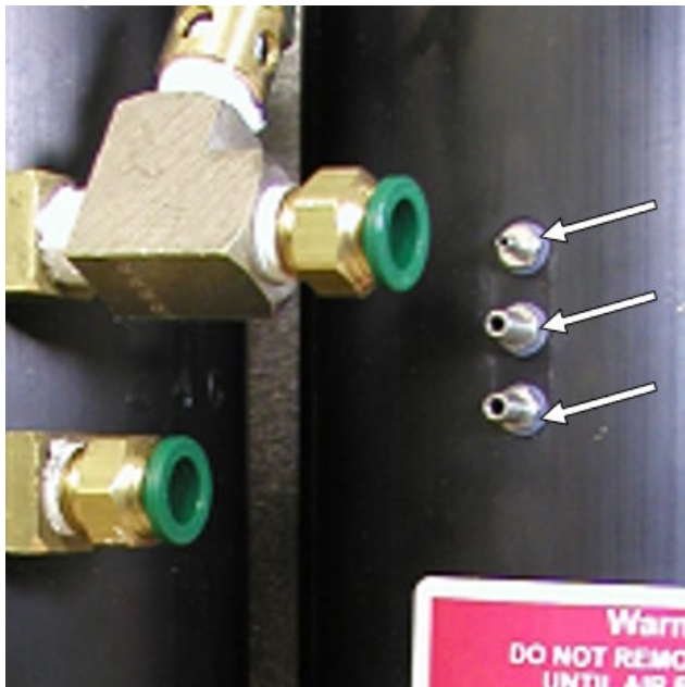
Fig. 5 Remove barbs on air tank
