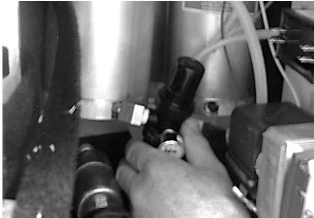
Fig. 3 Grasp regulator and pull out of air tanks.
